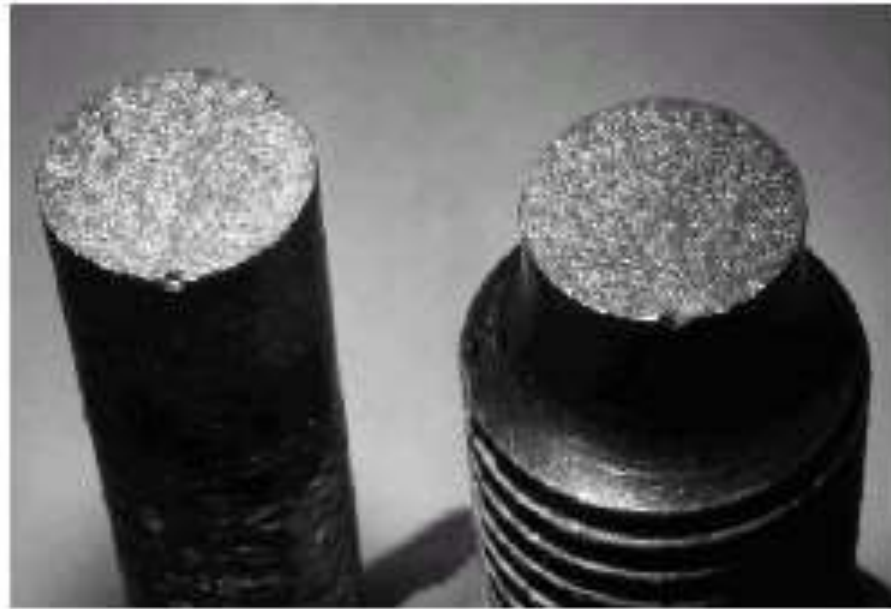
Brittle fracture in a mild steel
