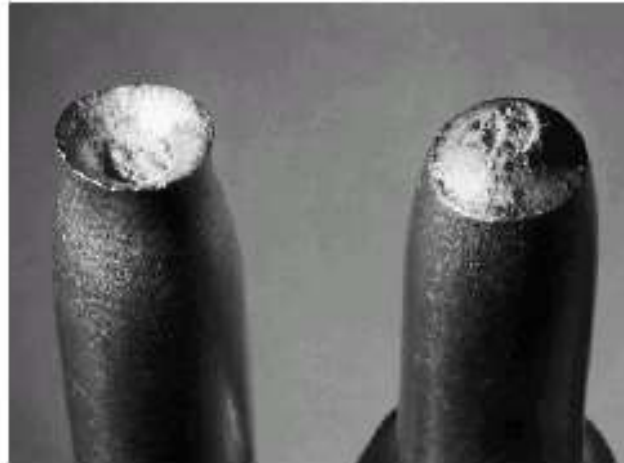
(Cap-and-cone fracture in Al)
